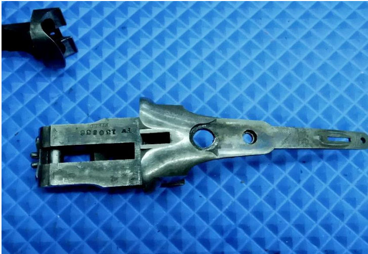
The action has taken a quite a beating over the years so it needs polishing before inleting into the stock.
