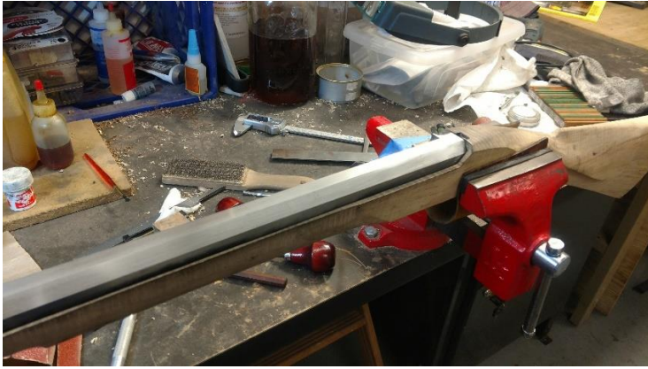
Here are a couple of photos of the Hawken three quarter stock .50 cal rifle. It has just a couple of millimeters left to complete the barrel channel inleting. Next will come the inleting for the tang and lock mortise
